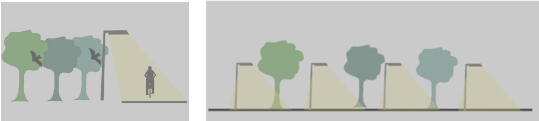
Luminaires to be mounted at short column and have a good optical light distribution.
